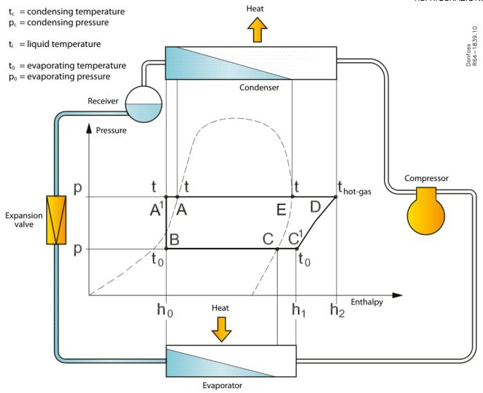
The condensed refrigerant in the condenser is in condition A which lies on the line for the boiling point of the liquid. The liquid has thus a temperature t c, a pressure p c also called saturated temperature and pressure.
